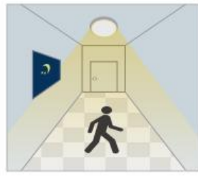
With insufficient ambient brightness, light dims to 100% when motion detected.
