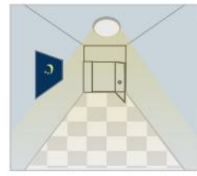
Light dims to standby level if no motion detected after holdtime.
